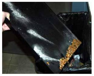
This photo shows the crumb tray partially removed. It is full of debris that should be disposed.
