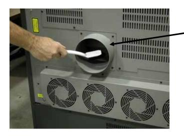
Periodically remove the duct from the back of the machine and clean both exhaust ports.
