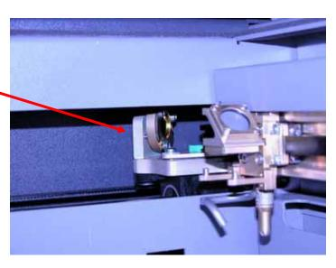
mirror is located in relation to the X-beam and carriage.
