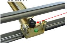
Press on the black spindle to slacken the belt
