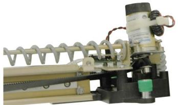
g. Replace the motor. Screw in the three captive screws.
