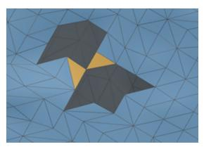
**Creased edges**: To remove creased edges according to the required angle set in the **Para**-meters.
