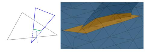
**Spikes**: To remove spikes. It is possible to adjust the level in the <u>Parameters</u>. A spike is detected on a mesh when there is at least one triangle from a vertex with a very different normal, compared to a fixed threshold of 60 degrees.
