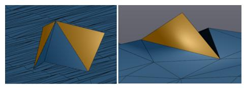
**Narrow bridges**: To remove small bridges between meshes. Threshold of the bridge width can be set.
