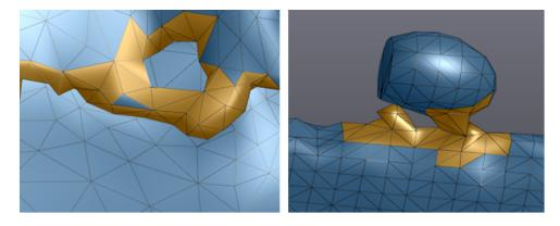
**Small holes**: To fill small holes. It is possible to adjust the *Max hole size* threshold in the **Parameters**.
