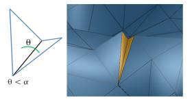
Narrow triangles: To remove narrow triangles (degenerated, compressed or slim).
