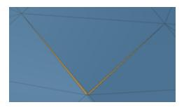
**Outcropping triangles**: Check this box option to remove outcropping triangles. An outcropping triangle has two edges on the mesh boundary.
