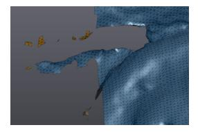
**Self-intersections**: To remove self-intersecting triangles. Self-intersections are found when a triangle is intersected by one (or more) other triangles. Then, both triangles are removed.
