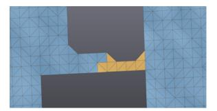
**Non-manifold triangles**: Count of non-manifold triangles detected in the mesh. This occurs when an edge is associated with more than two triangles.
