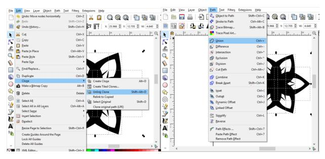
18. Now turn off the fill and turn on the stroke to turn the object into an outline that can be edge cut on the laser cutter by doing the operations below:
