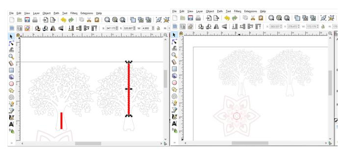
39. Finally, rearrange your pieces to fit within the board. Press "Ctr+A" to select all your pieces and go to "Stroke Style" under "Fill and Stroke". Change "Width" to 0.001 in, and your file is ready to be exported as a pdf for laser-cutting. Congratulations on making a 3D tree out of 2D slices of wood!
