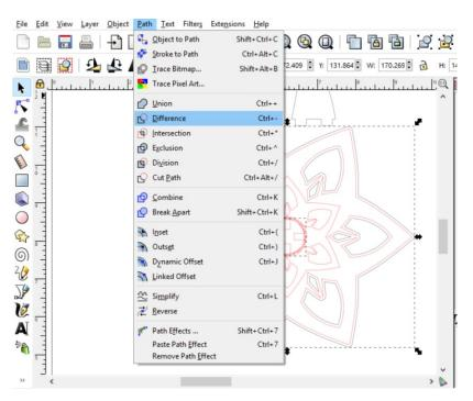
37. Now we want to make a slot to slide the halves of the tree together. First, make a copy of your tree. Then, create a rectangle with width of 4.9mm and a height a little more than half the height of the trunk. We will be using this to cut slots into each copy of the tree.
