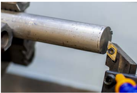
FIGURE 4.12: VERIFYING THE ZEROING ON THE STOCK.
