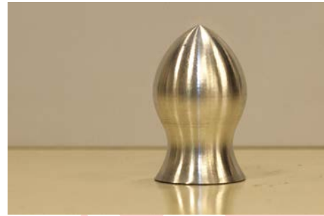
FIGURE 1.2: THE RESULT OF CREATING FIGURE 1.1 ON THE LATHE USING CAM OPERATIONS.
