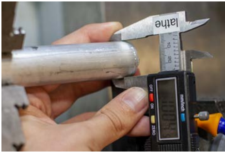
FIGURE 4.10: MEASURING THE DIAMETER OF THE STOCK.
