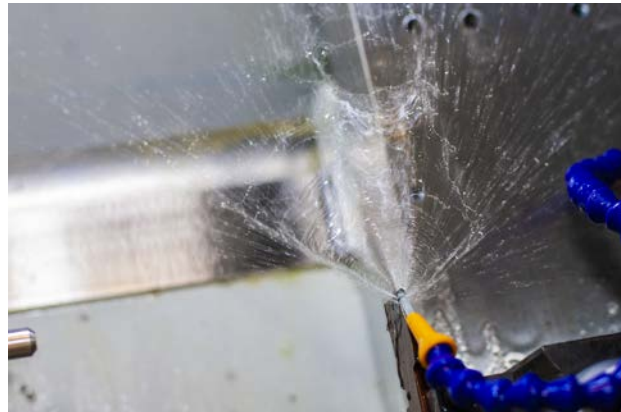
FIGURE 5.5: VERIFYING THE COOLANT SPRAY FOR TOOL 52.
