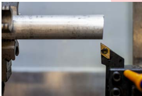
FIGURE 4.8: TOOL 51 READY TO APPROACH THE OD FOR ZEROING.
