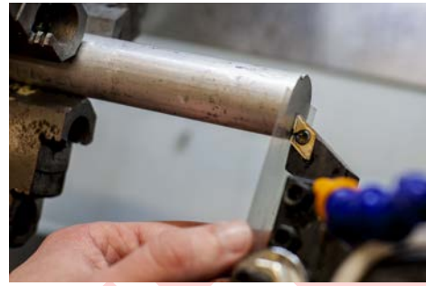
FIGURE 4.6: PINCHING THE FEELER TO THE FACE OF THE STOCK.
