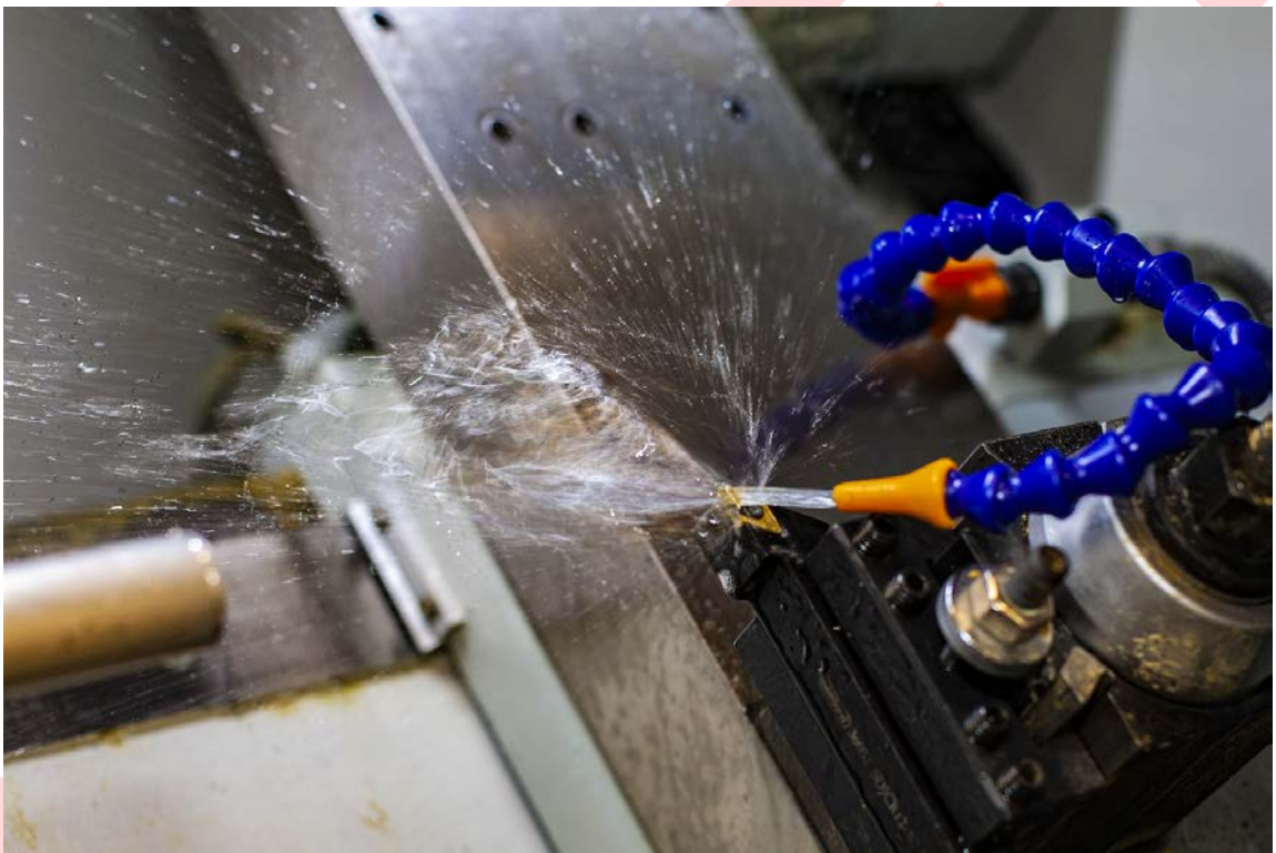
FIGURE 4.15: APPROPRIATE COOLANT SPRAY FOR TOOL 51.
