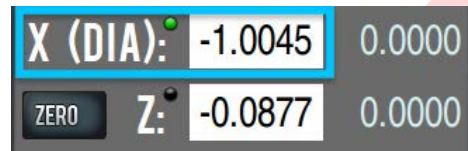
FIGURE 4.11: ZEROING THE X-AXIS.
