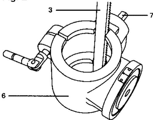
7. Slide the table support assembly with the rack (6, 7, 3) together onto the column support (10).
