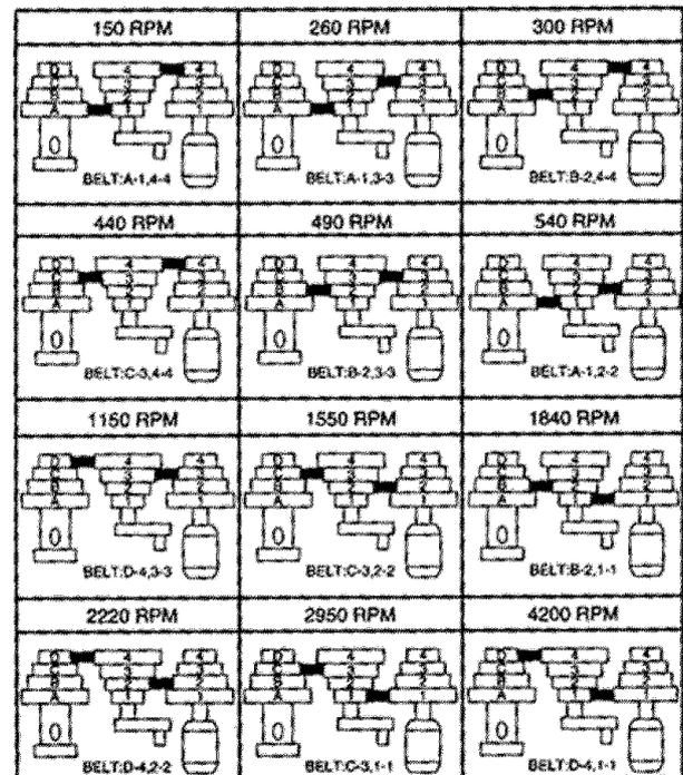
**DRILL SPEED RPM (FIG. Y)**
