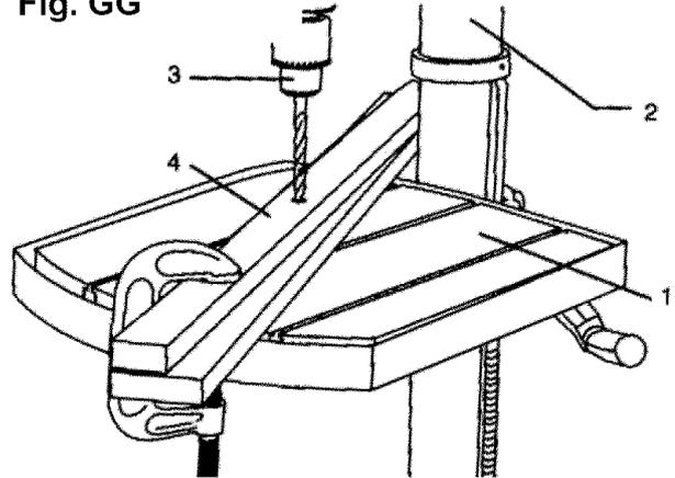
3. For small pieces that cannot be clamped to the table, use a drill press vise (optional accessory).
