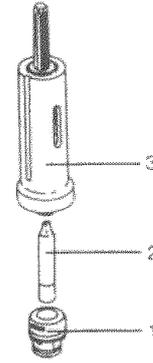
3. (FIG. M) Push the chuck (1) onto the spindle arbor (2). Tap gently to ensure seat.
