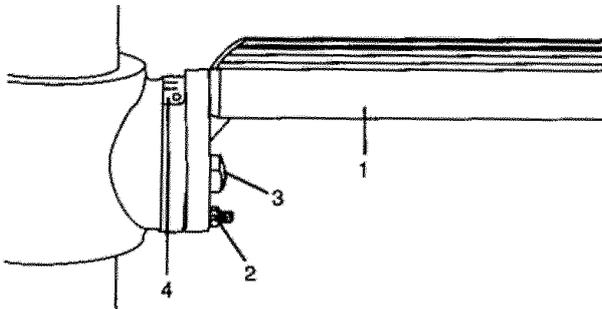
3. Tilt the table, aligning the desired angle measurement to the zero line opposite the scale (4). Tighten the bevel locking bolt.
