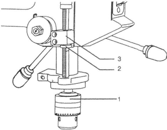
**REMOVING CHUCK AND ARBOR (FIG. FF)**
