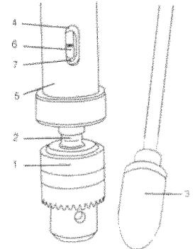
7. (FIG. N) Using a rubber mallet, plastic-tipped hammer, or a block of wood and a hammer, firmly tap the chuck upward into position on the spindle shaft.
