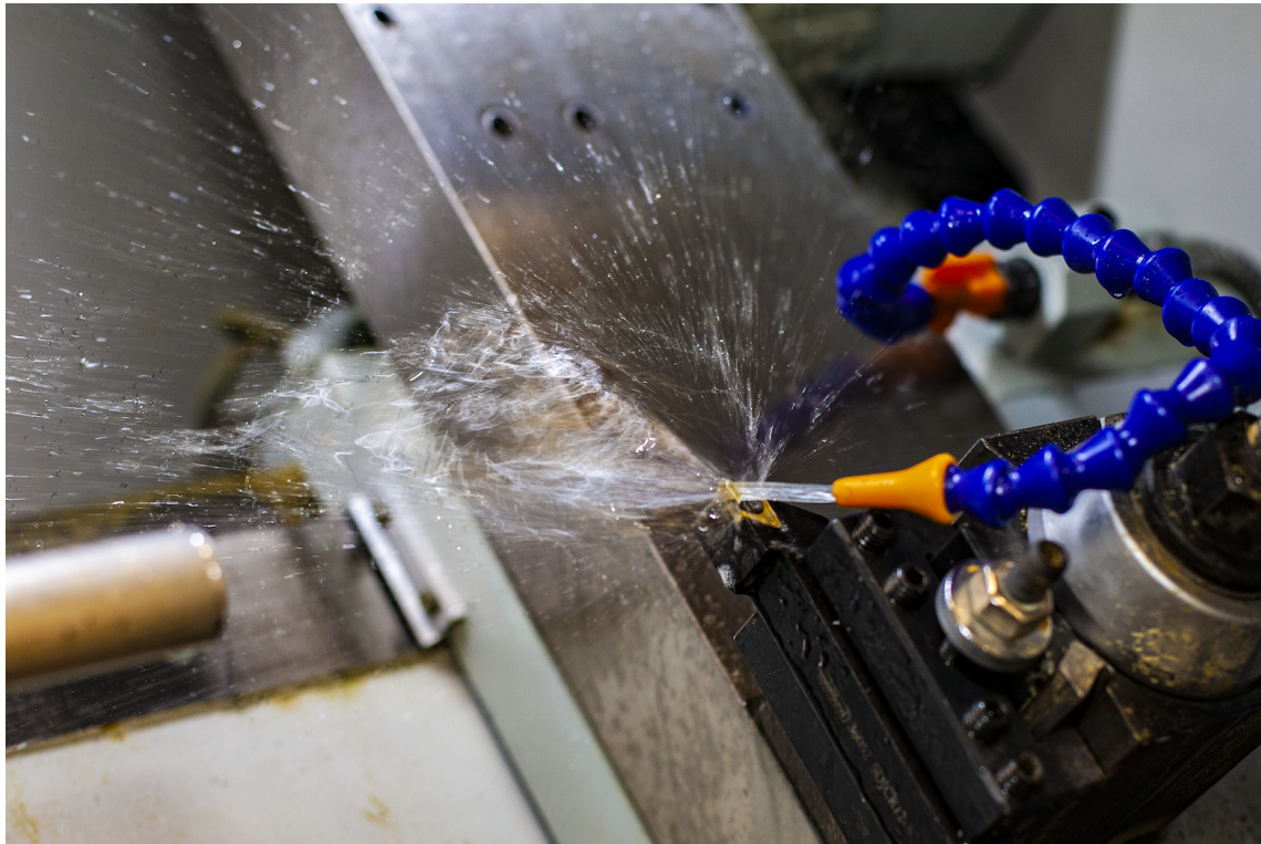
FIGURE 4.15: APPROPRIATE COOLANT SPRAY FOR TOOL 51.
