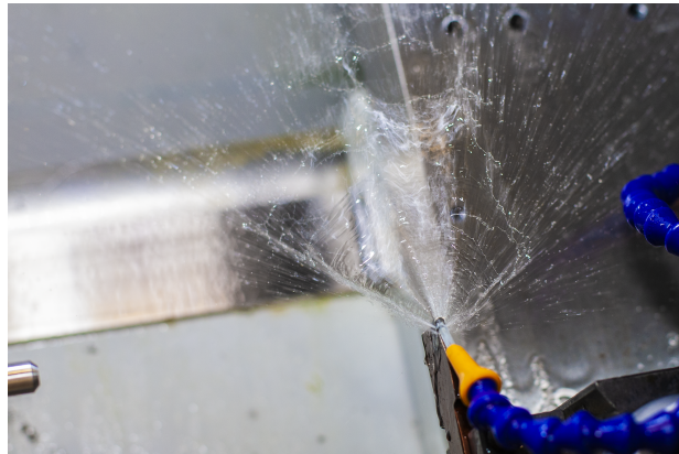
FIGURE 5.5: VERIFYING THE COOLANT SPRAY FOR TOOL 52.
