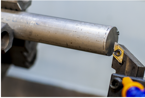
FIGURE 4.12: VERIFYING THE ZEROING ON THE STOCK.
