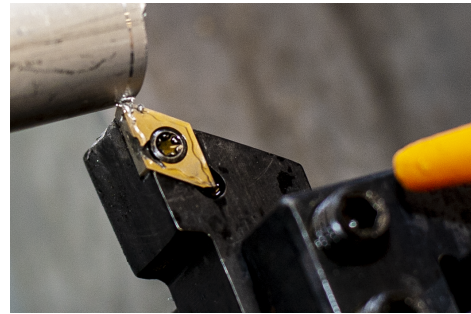
FIGURE 4.9: A FAINT CURL APPEARING AT THE TIP OF TOOL 51.
