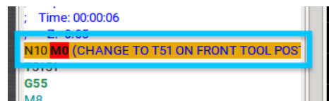
FIGURE 5.2: THE HIGHLIGHTED G-CODE INDICATING THE FIRST REQUIRED TOOL.
