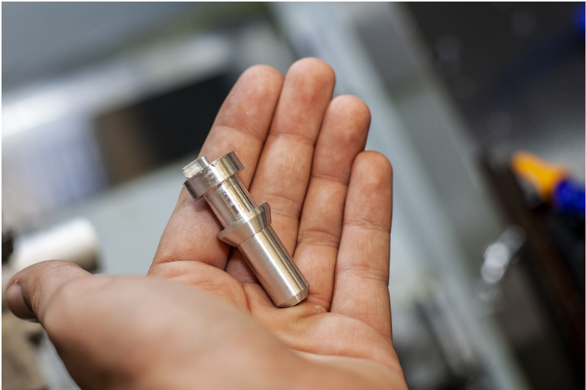
FIGURE 5.6: THE FINAL PIECE AFTER PARTING.
