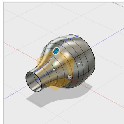
**Step 10:** Change the Revolve settings. Let's change the settings in the Revolve settings to change the **Angle** the direction that the curve is revolved.
