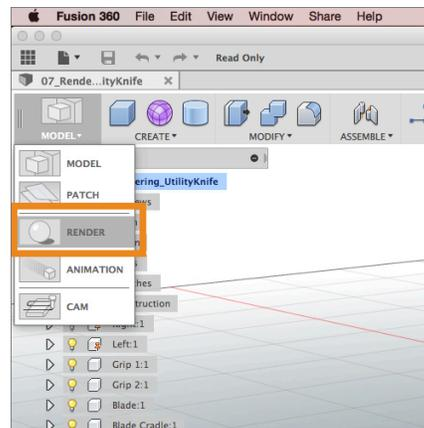
**Step 2:** Apply Materials to Geometry - Now that the model is in the Rendering Workspace you can begin assigning **appearance materials**.
