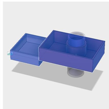
**Step 13:** Use joints to control the position of the cylinder.
