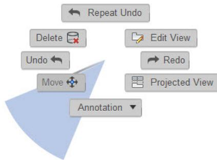
As you move the cursor from the center of the marking menu towards a command, its wedge highlights. Clicking anywhere in the wedge launches the command.
