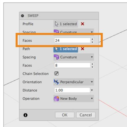
**Step 14:** Change the sweep orientation. There may be instances where the orientation of the profile as it moves along the path will give you a more desirable result. Use the **Orientation** option to change the sweep behavior.
