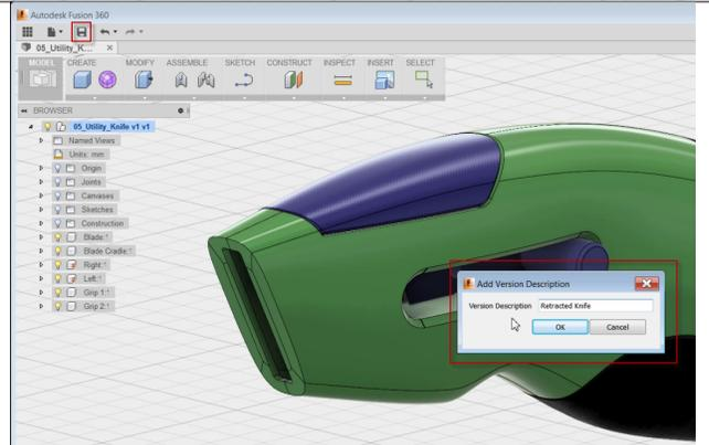
**Create a referenced document:** In this section, you create a drawing from the utility knife. Fusion maintains the relationship between the design and the drawing.
