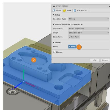
**Step 8: – Orientate and Locate the Work Coordinate System (WCS) correctly.**
