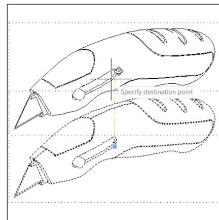
Move your objects around your drawing so they are nicely spaced, leaving the top right of the drawing space open (for a Parts List, to be added later).
