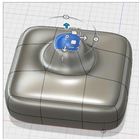
Note: You can use this hotkey function to extrude any edge(s) or face(s) that are selected on a T-Spline form.
