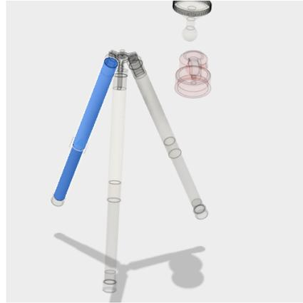
**Step 5:** Add a joint to the bottom end cap.
