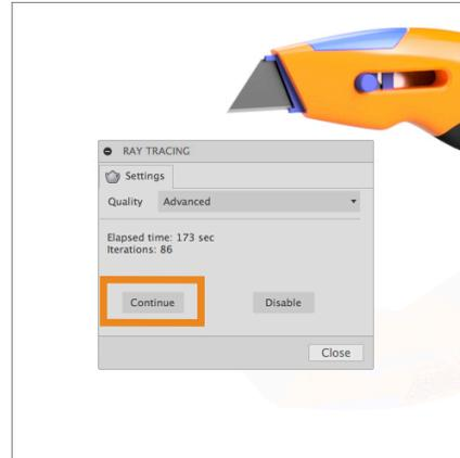
**Step 4: Start the Ray Tracer and Capture an image.** When rendering locally you manually capture an image when you are satisfied with the look of the image. All local **Ray Tracer** images will be based on the size and resolution of your screen.
