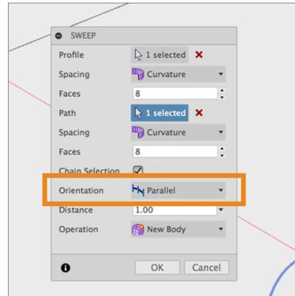
**Step 15:** Change the sweep distance. The Sweep command allows you to alter the amount of the path curve that is used to create the T-Spline form.
