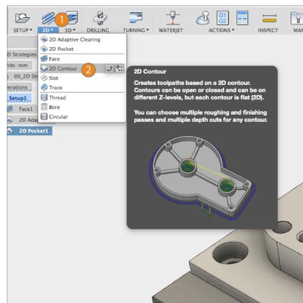
**Step 25:** – Select correct **TOOL** and **GEOMETRY**.
