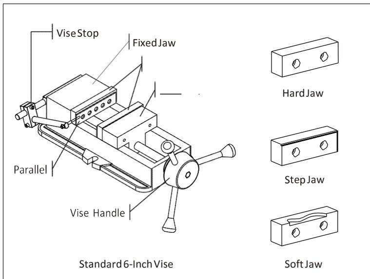
The **Fixed Jaw** remains stationary. The **Moving Jaw** opens when the **Vise Handle** is turned. It is a good practice to remove the vise handle after the jaws are closed and before running the program. This is done by simply sliding the handle off.
