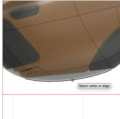
**Step 10:** Use **Edit Form** to move faces and edges until you have matched the T-Spline body to the profile of the Knife image.
