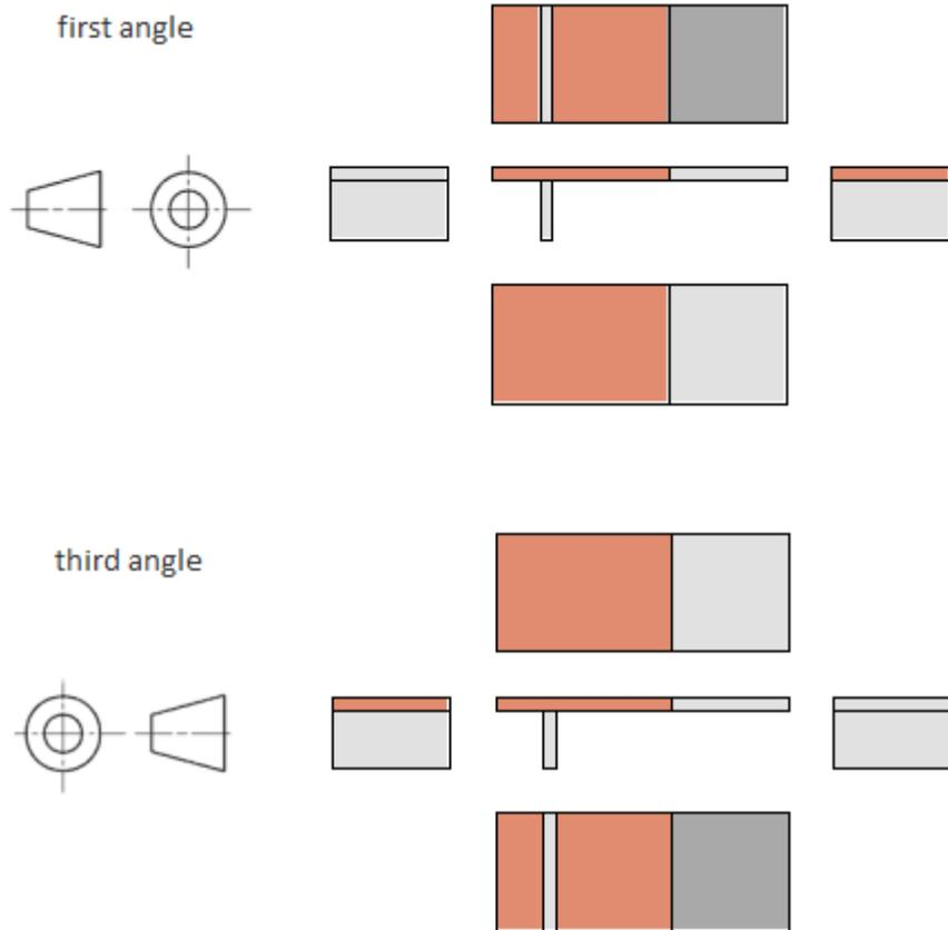
**First Angle Projection** – When you use first angle projection, projected views placed to the right of a base view depict the appearance when viewing it from the left. Projected views placed below the base view depict the appearance from above. The ISO drafting standard specifies that drawings use first angle projection. **By default, when the drawing format is set to ISO, the Drawings workspace will use first angle projection.**
