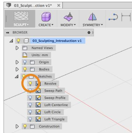
**Step 9:** Revolve a T-Spline using the sketch curve as input.
