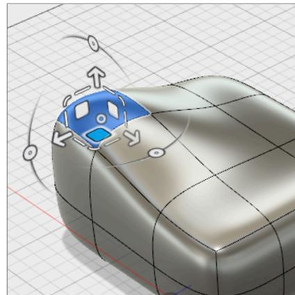
**Step 6:** Move a T-Spline edge and vertex.
