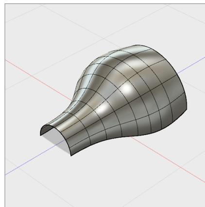
**Step 11:** Create a T-Spline Form using **Sweep**. The **Sweep** command uses two sketch curves to define a shape. One curve is selected as the **Profile**, which is swept along a **Path** curve to create the shape.
