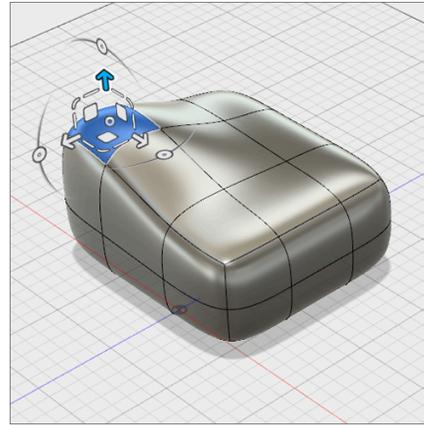
**Step 5:** Move a face in a planar direction.
