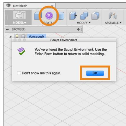
**Step 2:** – Select the T-Spline Box primitive
