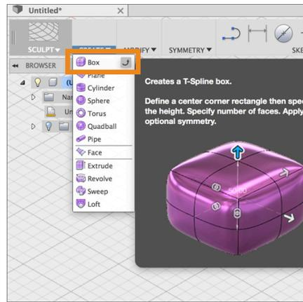
**Step 3:** Position the Box – When you create a new primitive you first need to indicate which plane you want to build on and then enter the dimensions of the primitive.
