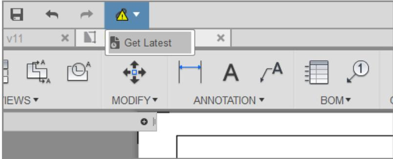
If any annotations associated with the drawing view geometry get disassociated because of the model change, badges are displayed on the screen. To delete or manually re-associate these badged annotations to the view geometry, you can snap to specify the points or select the objects you want the dimension to get re-associated.
