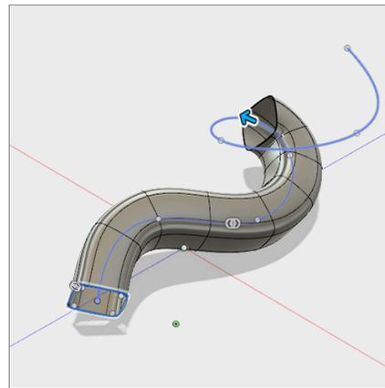
**Step 16:** Create a T-Spline Form with **Loft** using 3 sketch profiles as input to create a lofted shape.
