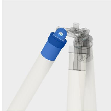
**Step 8:** Add joints to connect the legs to the bracket.
