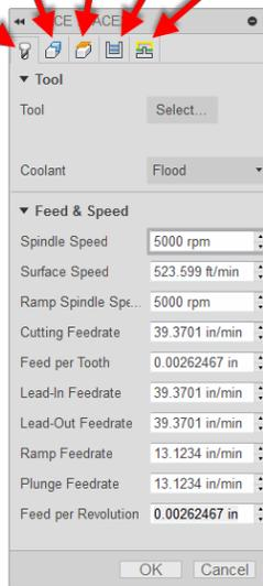
**TOOL TAB**– Defines the tool being used; as well as the feeds and speeds
