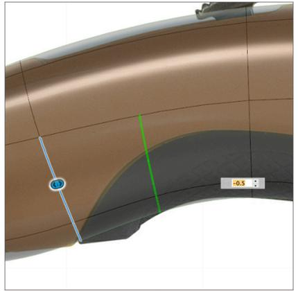
**Step 7:** Insert additional edges with **Insert Edge**.
