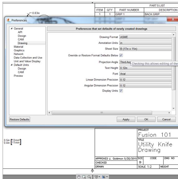
Note: The default settings are applied whenever you create a **new** drawing. Some of the settings can be modified after you have created a drawing, but settings like Drawing Format, Units, and Projection Angle cannot be modified once a drawing is created. If you need to switch these, you will have to create a new drawing.
