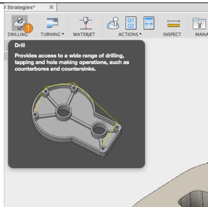
**Step 31:** – Select correct **TOOL** and **GEOMETRY**.
