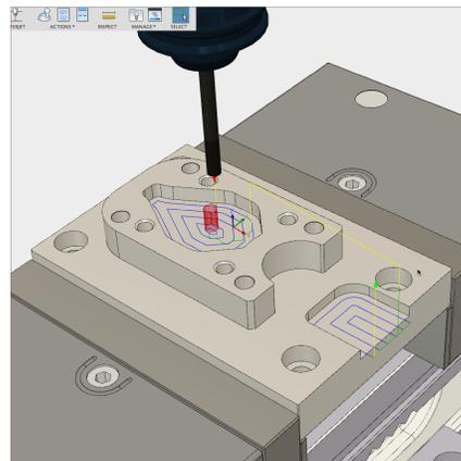
**Step 24:** – Apply a **2D Contour** Operation for a finishing pass.
