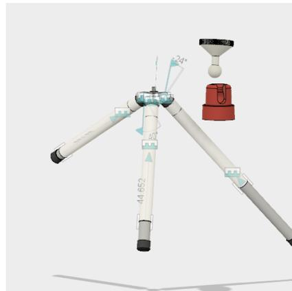
**Step 10:** Use the Joint command to join the red stand to the bracket.
