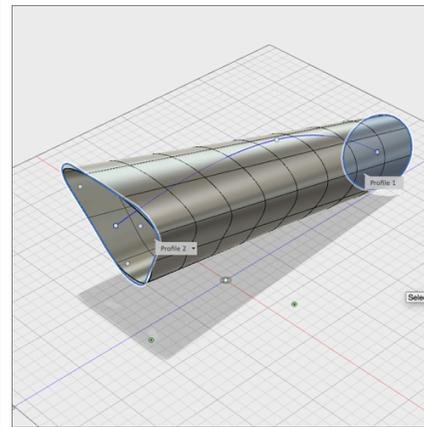
**Step 18:** Change the Loft shape by defining a centerline. By default the loft will always create straight transitional surfaces between profiles. To control the direction of the surface between the profiles you can add a sketch curve a centerline.
