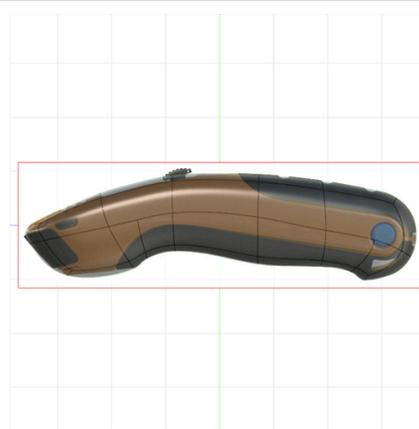
**Step 9:** Use **Insert Point** to draw edges on a face. To insert the final two edges we need, we'll use the **Insert Point** command. Slightly different from **Insert Edge**, the **Insert Point** command will easily insert an edge by connecting two points together.
