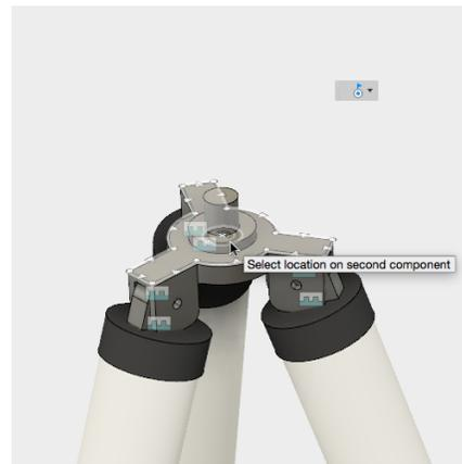
**Step 11:** Use the Joint command to join the stand and the camera mount.
