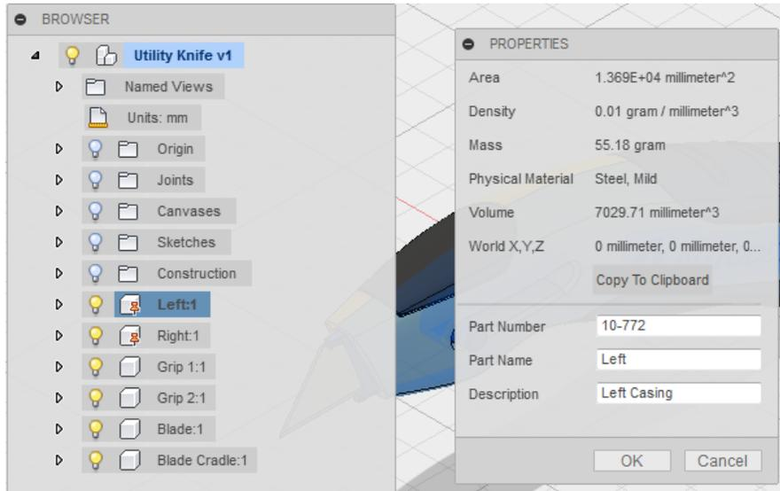
If you change the name or properties of a component in the Model workspace, the changes will be applied to the drawing once you associate the drawing with the saved model (see [Associatively Update the Drawing](#)).
