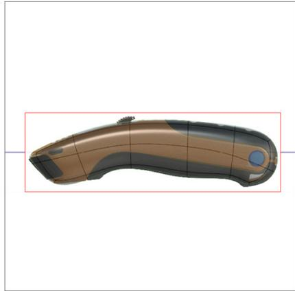
**Step 6:** Insert edges to get closer to the knife shape. Our T-Spline form is starting to resemble our reference image but there aren't enough edges in the T-Spline to capture all the detail of the Knife.
