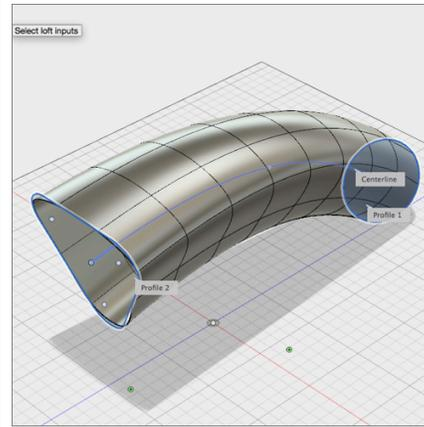
**Step 19:** The T-Spline surface is not matching well to the triangle profile. Let's increase the number of faces to improve the match.
