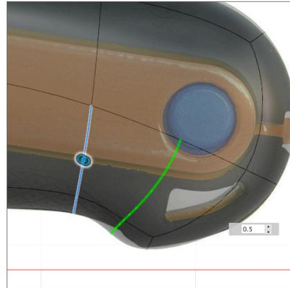
**Step 8:** Move the inserted edges with **Edit Form**.
