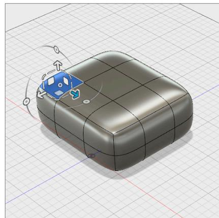
**Step 4:** Move a face in a single axis direction.
