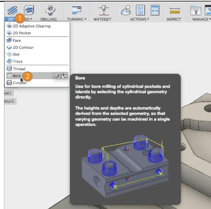
**Step 28:** – Select correct **TOOL** and **GEOMETRY**.
