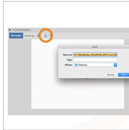
**Step 5:** Create a cloud render using Named Views. The cloud renderer automatically creates small sized rendered images based on the **Top, Front, Right** and **Home** named views every time you manually save a new version or an auto save is done. If you want to create automatic Cloud Render images of a specific view you can create a new named view to accomplish this.
