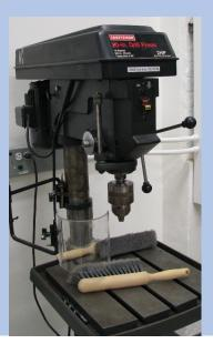
The precision press is used for cutting precisely measured holes using the movable bed.
