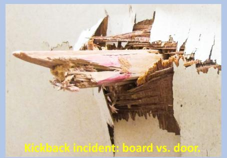
This board was flung through an interior door when the saw blade snagged it and caused kickback. Imagine if the operator had been in the way of the projectile.
