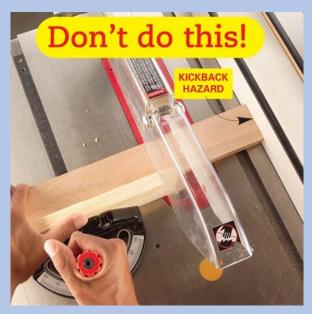
Above, a hazardous situation has been created by using both the fence AND miter gauge to guide a board through the cut.
