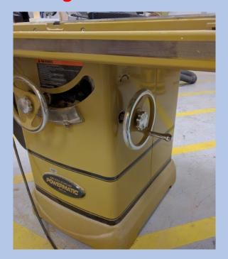
There are two handwheels on the saw. The handwheel on the front face (where the operator stands) adjusts the blade height. The knob inside of the handwheel locks the chosen setting in place.
