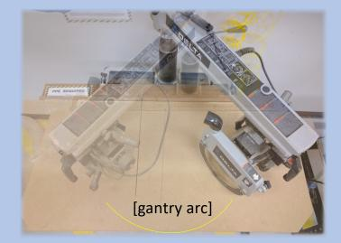
The powerhead can be raised and lowered using the arm. It can also change blade angle relative to the table, and rotate perpendicular to the gantry.
