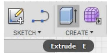
extrude the toothpaste into a 3D cylinder. Click on the Create menu and Extrude tool will be activated. Then click anywhere in the circle to select it. An arrow will appear along with the extrude menu.
