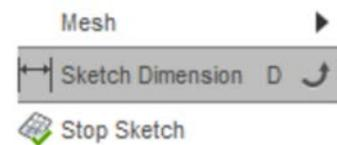
Click anywhere and set the dimension to a value of 0.2 in. Repeat this step with the bottom side of the rectangle. This locks the lower right corner relative to the origin, but the lengths of those sides can still be changed. Next, dimension just the bottom side to be 0.4 inches and then separately dimension the right side to 0.4 inches as well to make it square.
