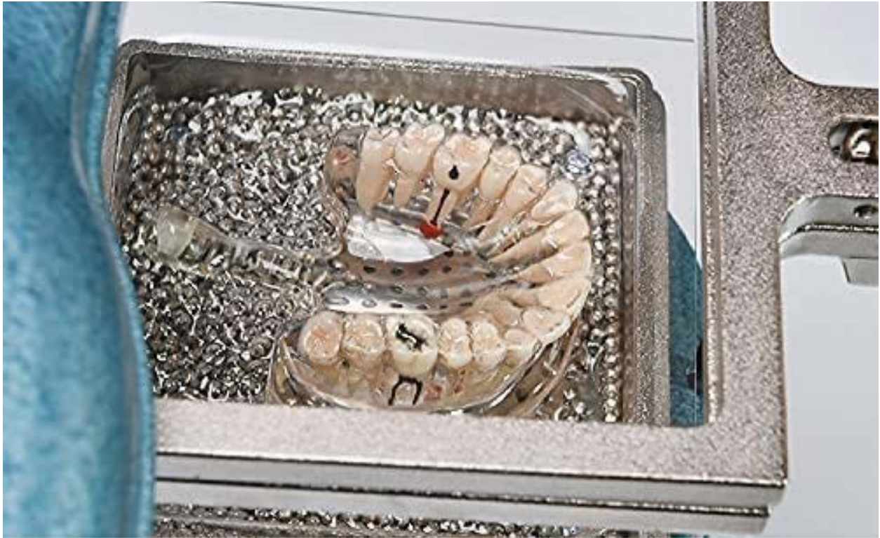
Figure 5: Example of a dental model placed on the steel ball tray for vacuum forming.
