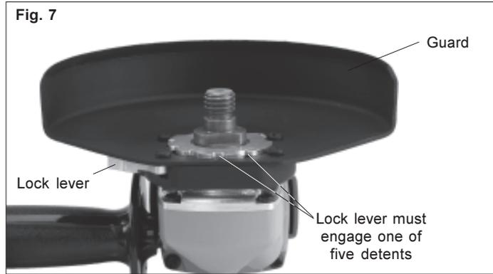
This tool is shipped without the guard installed. The guard must be used when using the tool as a grinder. The guard should be removed when using tool as a sander.
