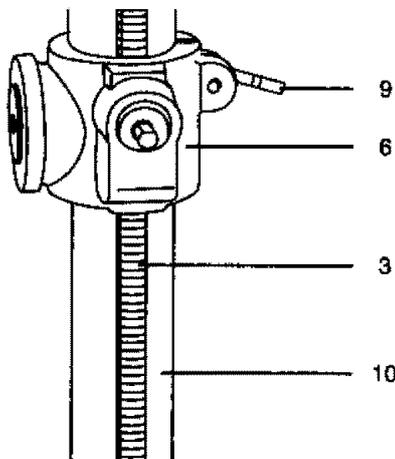
9. Install the collar (2) to the top end of the rack (3) on the column (10). Tighten the set screw (1).
