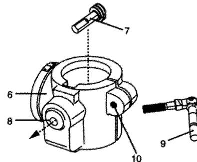
6. Place the rack (3) in position inside the table support (6), making sure the worm gear (7) on the inside of the table support is engaged with the teeth of the rack.
