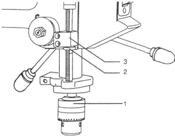
**REMOVING CHUCK AND ARBOR (FIG. FF)**
